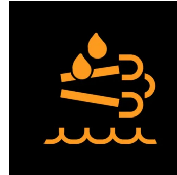
Selective Catalytic Reduction (reduces \text{NO}_x with DEF)
